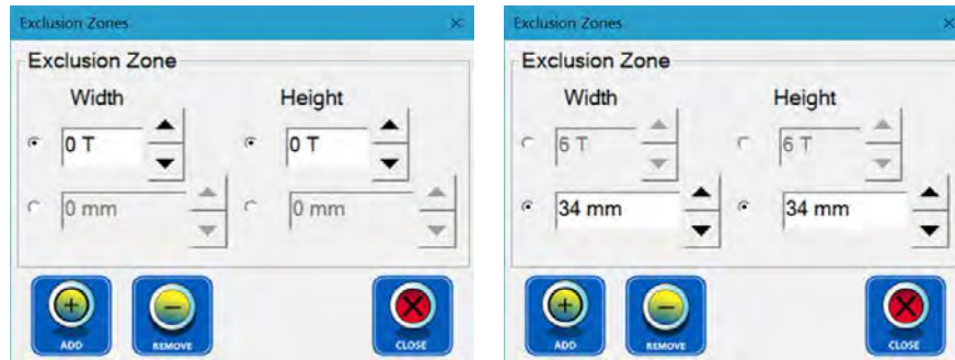
Using Wall Thickness
